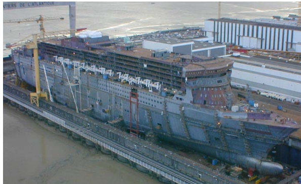
Fig 14: Cruise ship construction in a floating dock and structural arrangement of a cruise ship.
