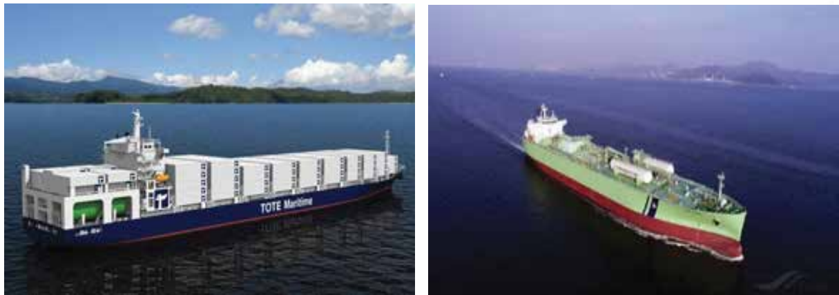
Fig. 2 (a) World's first LNG powered containership Isla-Bella 7 (b) World's first LPG powered ship BW GEMINI 8
