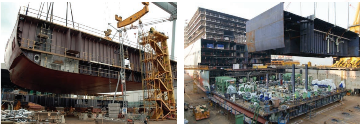
Fig 13: Block or modular construction
