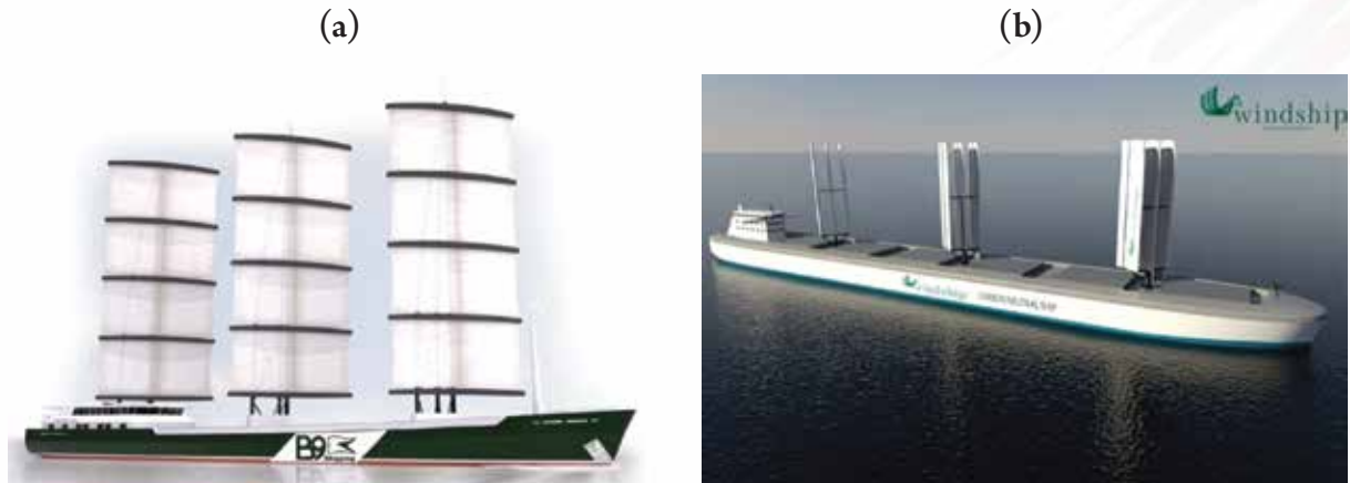
Fig. 3 (a) B9 cargo ship with soft sail 12 (b) Windship with rigid sail 13
